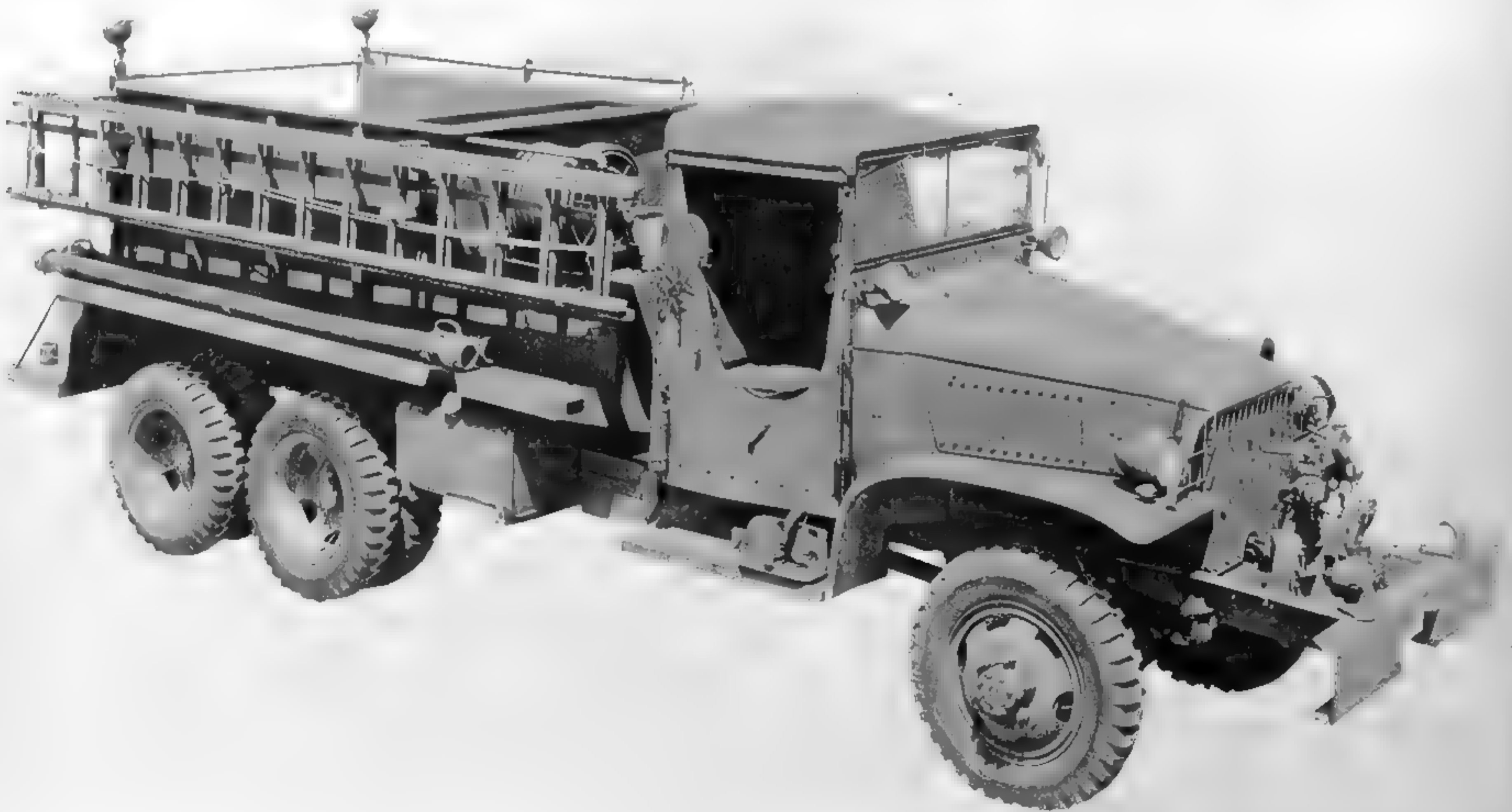
The military class 335 and 530 fire trucks were conversions done by the military on CCKW chassis. The conversion involved both the mounting of a conversion kit and the cannibalization of a class 325 4x2 fire truck. (Photo courtesy of United States Army Engineer School History Office).
